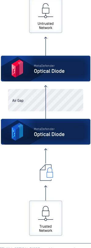
NETWALL OPTICAL DIODE provides one way data transfer using an optical link
