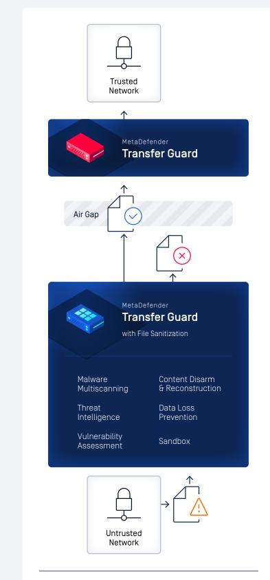
SUPER NETWALL provides one way data transfer with additional file sanitization by MetaDefender Core
