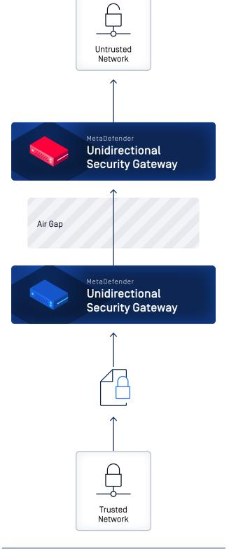
METADEFENDER USG provides one way data transfer over a serial connection
