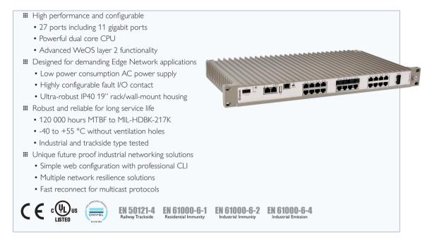
The RFIR (RedFox Industrial Rack) is a high performance layer 2 industrial Ethernet switch designed for high network traffic applications. Various port configurations are available that can be further customised with SFP transceivers. RFIR is powered by the Westermo WeOS network operating system.
